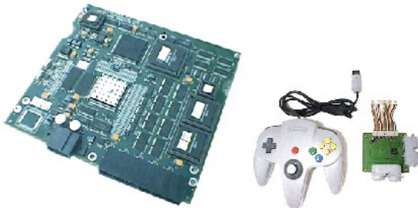
4. Figure 5-1-1 The N64 emulator board, the controller and the conversion adapter
